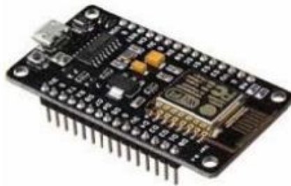
Figure 2: NODE MCU Development board
