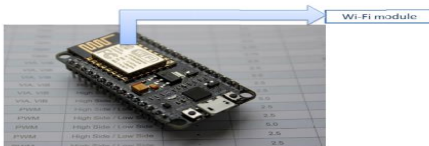
Figure 3: NODE MCU with inbuilt wifi module
